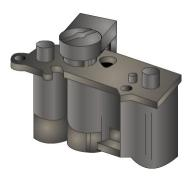
The RCM uses the hall effect signal of the SPS to determine the drivers airbag deployment rate.
