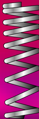
Typical Variable Rate Coil Spring (Should be installed with the tight coils up as depicted here)
