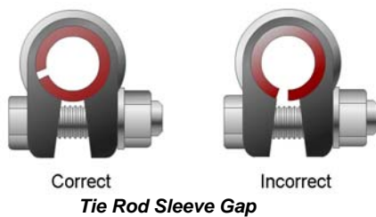
Tie Rod Sleeve Gap
