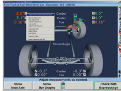
Camber and other angles are displayed on the screen. (Courtesy of Hunter Engineering)
