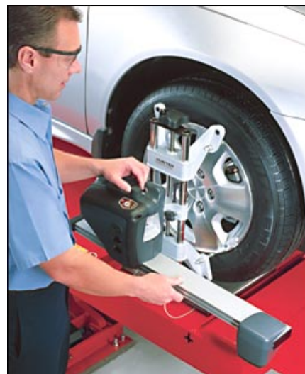
Alignment sensor and clamp adapter (Courtesy of Hunter Engineering)
