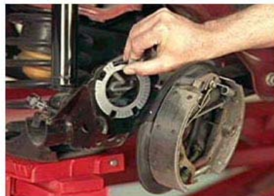
Installing a rear shim
