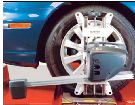
The component on the left of this sensor projects a toe signal across to the sensor on the opposite wheel. It receives a similar signal in return, and the left rear sensor projects a signal forward to this sensor. (Courtesy of Hunter Engineering)
