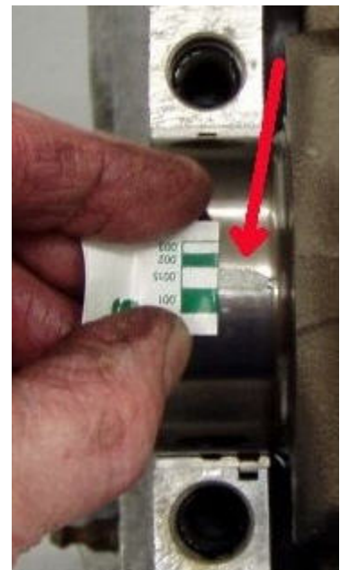
Bearing Clearance Measurement
