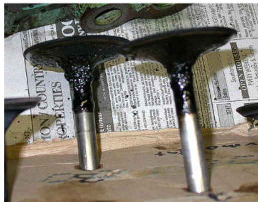
Carbon Deposits on Intake Valve
