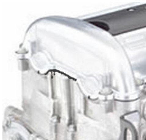
Using Foot Powder for Visual Leak Detection
