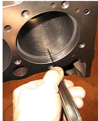
Measuring Piston Ring End Gap
