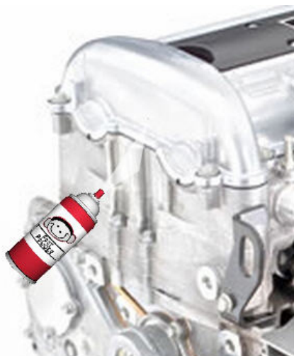
Using Foot Powder for Visual Leak Detection
