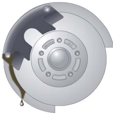
(fig. 61) The bottom of the caliper will be damp with fluid if a disc brake is leaking.
