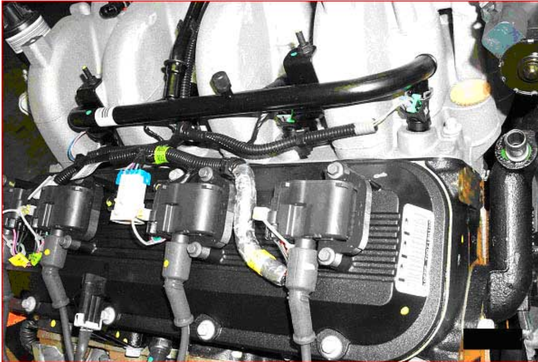
On this one-coil-per-plug system, the coils are mounted on the valve covers. Note the fuel rail located above the valve cover.
