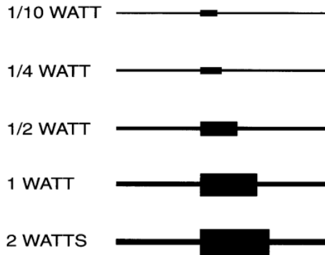
Figure 3-13 Resistor sizes by watts
