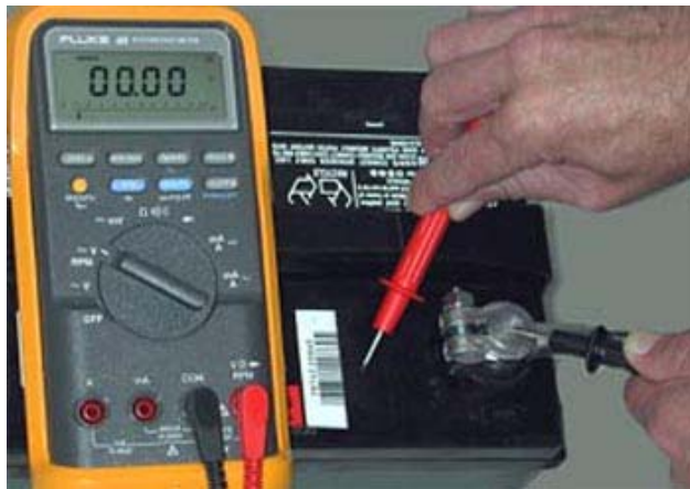
Checking for Electrical Leakage
