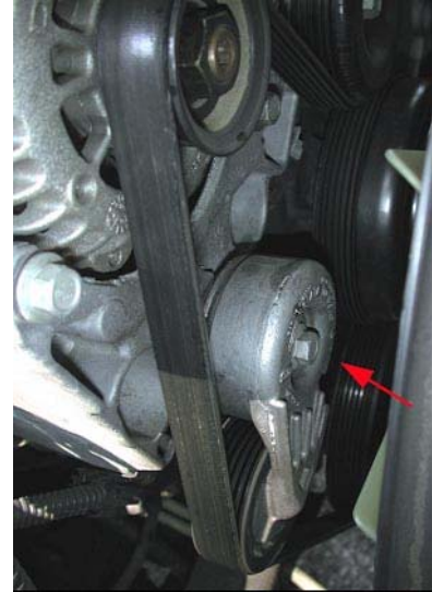
This system uses a flat, serpentine belt with a self-tensioner. A spring inside the unit applies the proper tension to the belt.
