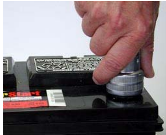
Cleaning Terminals with a Terminal Brush
