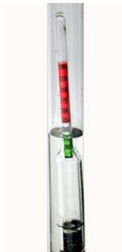
Notice how buoyant the float is in this fully-charged battery.
