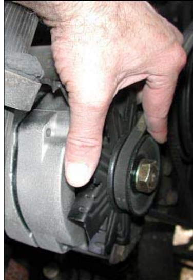
Checking for belt slippage
