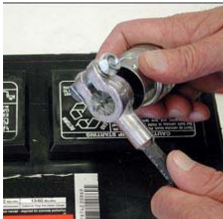
Cleaning Terminals with a Terminal Brush
