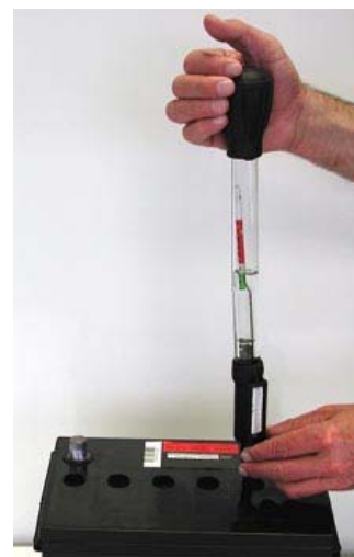
The next cell is checked, and also reads good: 1.265. But...
