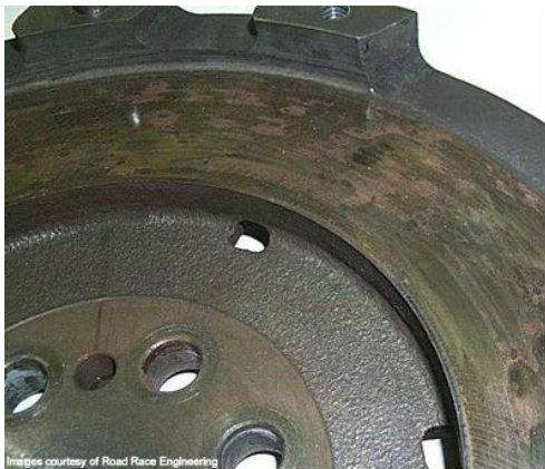
This flywheel has heat marks but can be resurfaced.
