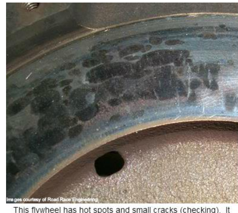
This flywheel has hot spots and small cracks (checking). It can probably be resurfaced.
