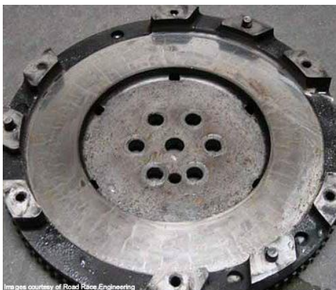
This flywheel has moderate to deep cracks. It is too thin to be resurfaced and will have to be replaced.
