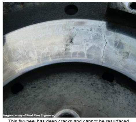
This flywheel has deep cracks and cannot be resurfaced.
